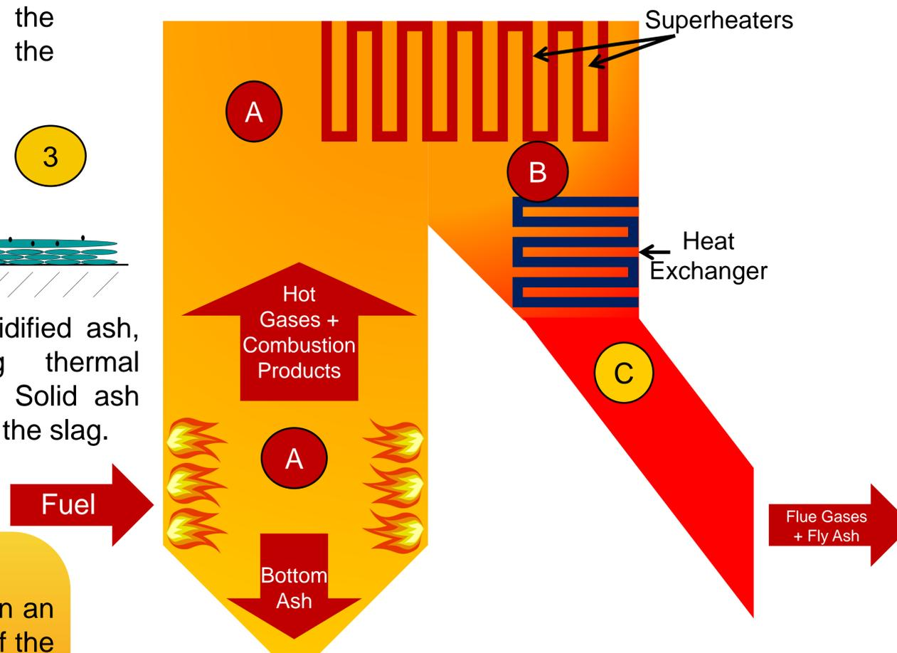
Simplified diagram of a typical pulverised fuel boiler
