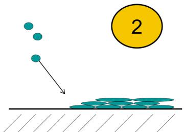
More sticky ash deposits on the solidified ash, building the deposit, increasing thermal resistance and surface temperature. Solid ash particles may be absorbed, thickening the slag.
