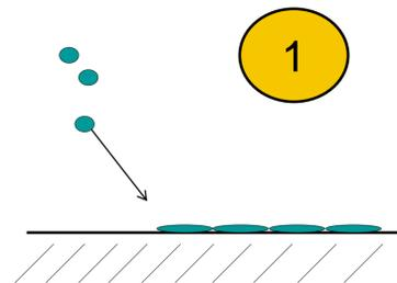
The molten/sticky ash is carried by the combustion gases. They impact on the cooler surfaces, solidifying.
