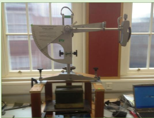
A section of tyre is attached to the end of a pendulum arm. When released, the arm swings down so the tyre can interact with a section of rail.
